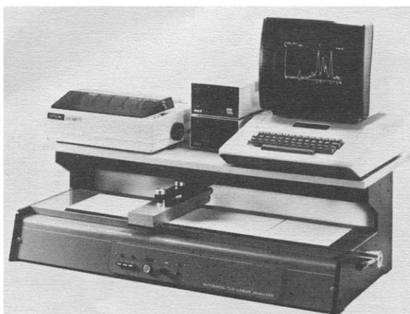
Figure 4 The Berthold LB 284 linear analyser and data system for the detection of radioactivity on TLC plates.
